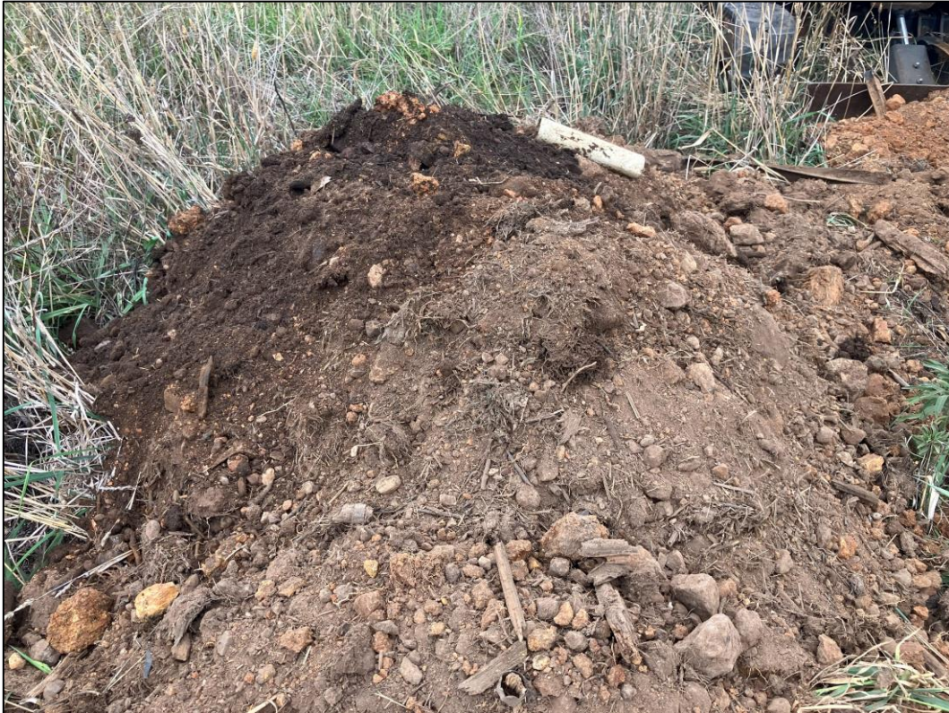
Site Photograph 13.1.2 View of silty CLAY fill material identified within 'TP05', located south of the main residence, as observed 3 March 2026.
