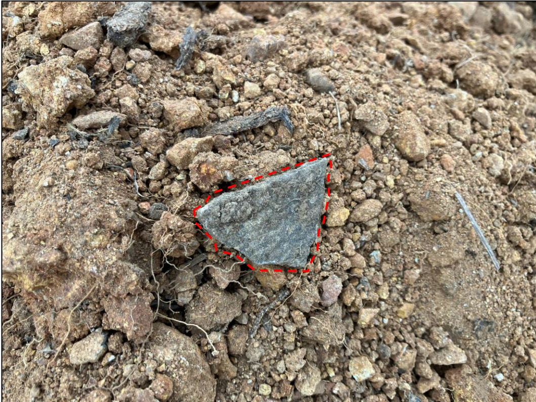
Site Photograph 13.2 Representative view of potential asbestos containing fibre cement fragment 'TP05-1.2-1.3-FC', as observed within 'TP05' on 3 March 2026.
