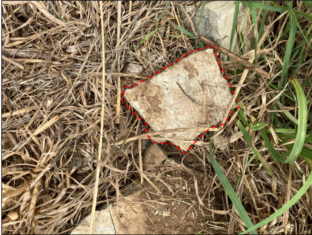
Site Photograph 5.5 Representative view of potential asbestos containing fibre cement fragment, as observed within on surficial soils south-east of the main residence, on 3 March 2026.
